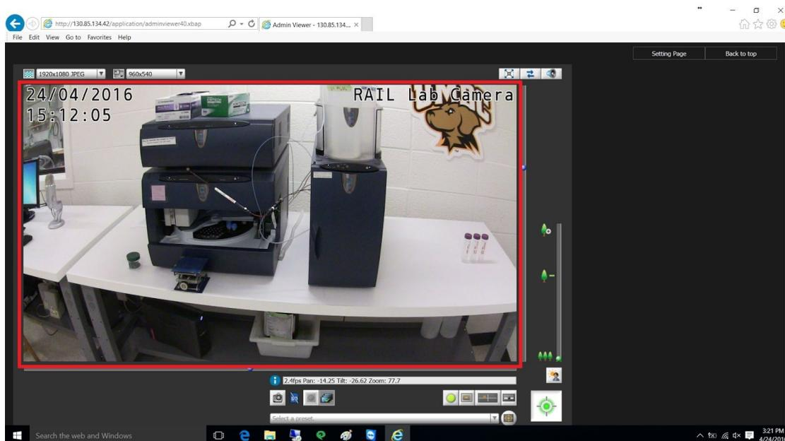
4. In order to zoom in and out on different parts of the instrument, use the panel on the right hand side window with the tree icons. You can make the camera window full screen by clicking on the first icon in the upper right hand corner.
